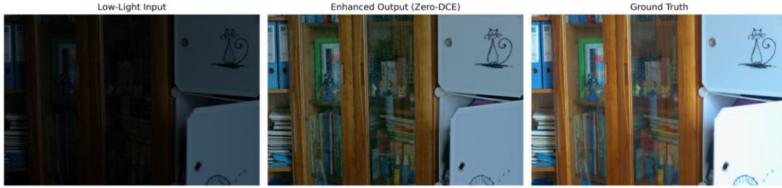
Figure 6. LOL benchmark visual comparison: low-light input, enhanced output generated by Zero-DCE, and the corresponding ground-truth normal-light image.
